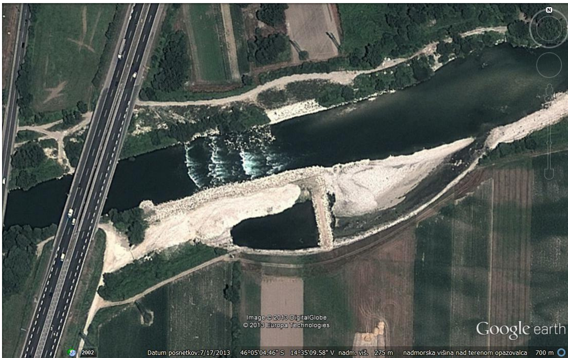
Figure 33: The riverbed ramp downstream of the Šentjakob highway Bridge after the Sava 2012 Flood. The flood caused a local right bank cut downstream of the ramp; the repair works have been already done (source: Google Earth, July 17, 2013).
