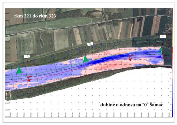
Figure 7. Proposal for the new positions of the floating signs at the sector Jaruge-Novi Grad
