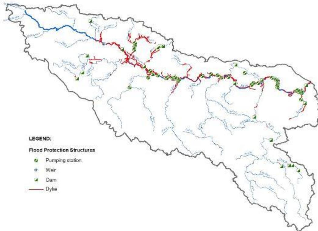
**Figure 8: Flood protection structures along the Sava River
