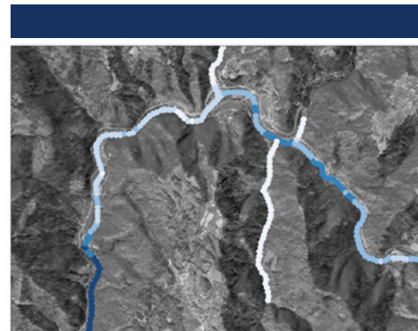
Draft model for watercourses assessment by their attractiveness for hydropower – darker colour indicates higher attractiveness
