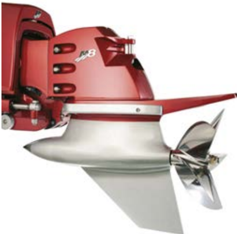
Figure 21 ◀ Arneson drive with partially submerged propeller on the end of the shaft movable in horizontal and vertical direction. The blackcuff protects the Cardan joint
