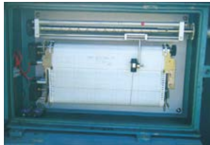
Figure 79 ► IA plotter recording the water stage on a paper tape - limnigram
