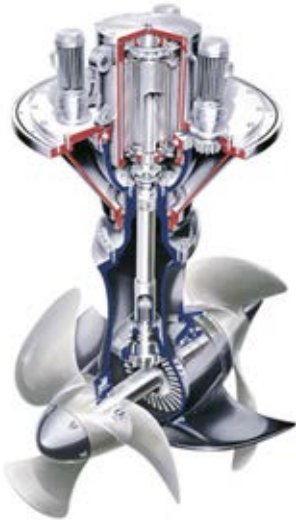
Figure 23 ▲ Azimuthing thruster, electrically driven with tandem propellers – SCD
